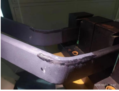
Fig. 1. Picture of an aging stator bar.
